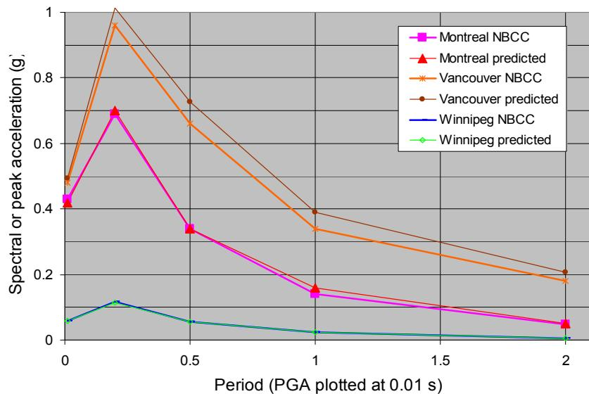
**Figure 3.** Comparison of NBCC and predicted (ratio-derived) UHS for Vancouver, Montreal, Winnipeg
