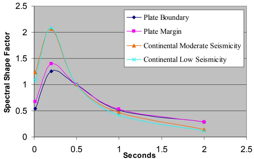
**Figure 2.** Spectral shape factors normalized at T=0.5 s (PGA is plotted at 0.01 s)
