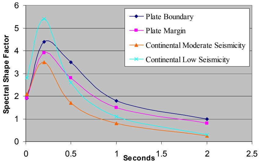
**Figure 1.** Ratio of (2%/50 yr Spectral and PGA) to 10%/50 yr PGA (PGA is plotted at 0.01 s)
